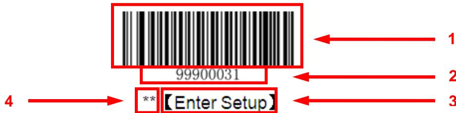
The figure above is an example that shows you the programming barcode and command for the Enter Setup function:
